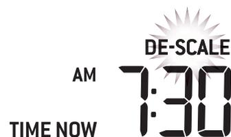
Remove the 'DE-SCALE' icon by pressing the SINGLE CUP and CARAFE button together, then follow these steps:
